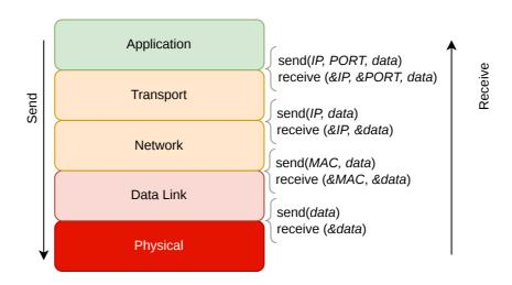
\*the initial TCP/IP stack did not make any difference between the *Physical* and the *Data Link* layers
